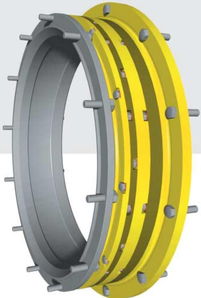
The air barrier chamber also functions as a damper of the dynamic hydraulic pulsations present in an aft sterntube seal. Pressure fluctuations inside the seal caused by radial and/or axial shaft movements, are cushioned. This makes the Airguard 3AS aft seal much less sensitive to the so-called pumping effect due to shaft vibrations as encountered in conventional seals.
